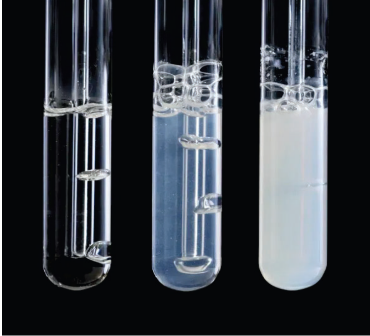
Figure 20: A well known experiment from reference [50] is to bubble human exhaled breath, which is about 4% \text{CO}_2 by volume, through limewater. The test tube on the left shows initially clear limewater, a subsaturated solution of \text{Ca}(\text{OH})_2 . The middle test tube is produced by the first few bubbles. It contains a sparse milky suspension calcite crystallites, \text{CaCO}_3(\text{s}) . Blowing still more bubbles makes the dense, milky suspension of the test tube on the right.
