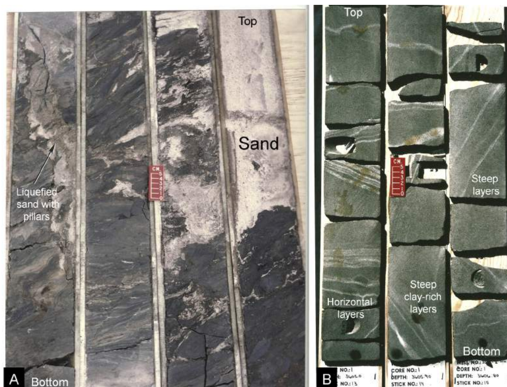
Fig. 11 A—Core photograph showing liquefied sand with a vertical pillar of sand (arrow) cutting across mudstone. Lower left is bottom and upper right is top. Pliocene, offshore Nigeria. Figure from Shanmugam (2012a) , with permission from Elsevier. Copyright Clearance Center's RightsLink: Licensee: G. Shanmugam. License Number: 3880791279258. License Date: June 2, 2016; B—Core photograph showing steeply dipping clay-rich layers (white) adjacent to horizontal layers in sandstone. Cretaceous, Agat Formation, offshore Norway. After Shanmugam et al. (1994) , reprinted by permission from American Association of Petroleum Geologists (AAPG).
