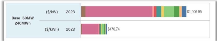
Figure 4: Cost details for utility-scale storage (4h 240MWh usable)
