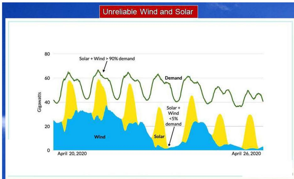
**Fig. 19.** Diagram showing showing unreliable nature of wind and solar energy sources that do not meet the demand. Note intermittent wind and solar can go to near zero for extended period of time. Diagram from Epstein (2022). Portfolio/Penguin.
